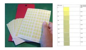
Test strips – simple and practical to attach to a web for approximate dose
